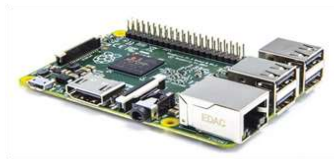
Fig. 1 Hardware of Raspberry Pi Model.
