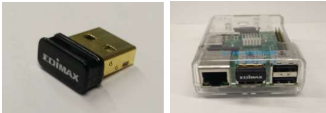
FIG 3. Raspberry Pi to WiFi adapter interface
